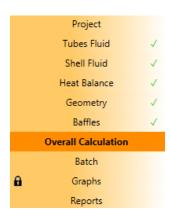
The green ticks indicate that **Tubes Fluid** and **Shell Fluid** are defined correctly, and the **Heat Balance** and **Geometry / Baffle** calculations are correctly done. The lock symbol next to **Overall Calculation** has disappeared meaning that this calculation can now be done. The lock symbol still appears next to **Graphs**, indicating that the **Overall Calculation** has not been successfully completed.
